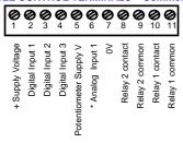
\* Analog inputs should be connected to terminals 6 & 7.
